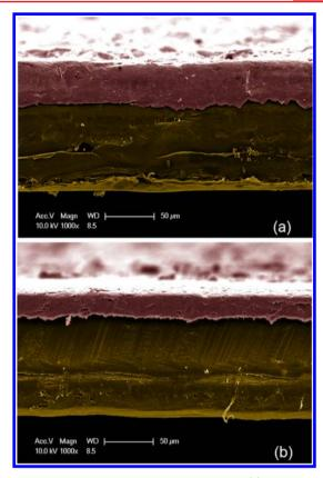
Figure 1. Cross-sectional SEM images of the (a) uncompressed (sample #1) and (b) compressed (sample #5) GL-on-PET. The pseudo colors are used to indicate the graphene laminate (burgundy) and PET (yellow) layers. The thickness of the shown GL layers is ~44 and 24  $\mu m$  for the uncompressed and compressed samples, respectively. The thickness of PET substrate is ~110  $\mu m$  for both compressed and uncompressed GL-on-PET. The laminate thickness variation is clearly seen from the micrograph.
