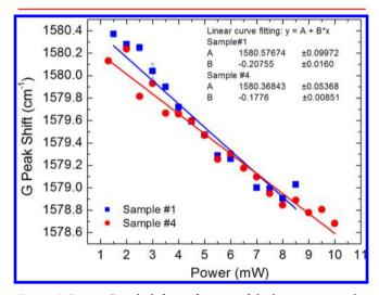
**Figure 6.** Raman G peak shift as a function of the laser power on the sample surface. The results are shown for the uncompressed (sample #1) and compressed (sample #4) GL-on-PET. The shift in G peak position with increasing power indicates the local temperature rise. The slope of these linear dependencies is used for the extraction of the thermal conductivity.
