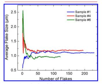
**Figure 3.** Statistical analysis of the FLG flake size in GL-on-PET samples. The calculated average flake size is shown as a function of the number of flakes taken into account. The data is presented for the uncompressed (sample #1) and two compressed (samples #4 and #6) GL-on-PET. Note that the flake sizes converge to the asymptotic average values of 1.10, 1.18, and 0.96 after the number of the accounted flakes exceeds about a hundred.
