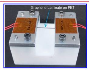
**Figure 4.** Optical image of the specially designed sample holder for optothermal Raman measurements with macroscopic thin films. The GL-on-PET sample under test (seen as gray ribbon) is suspended across a trench and fixed with two massive aluminum pads acting as the heat sinks. The ribbon is heated with the Raman laser in the middle. The experimental setup is a scaled up version of the original one used for the measurement of the thermal conductivity of graphene.
