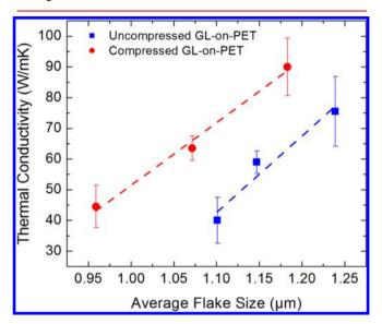
**Figure 7.** Thermal conductivity of GL-on-PET as a function of the average flake size *D*. The results are shown for the compressed (red circles) and uncompressed (blue rectangles) GL-on-PET samples. The dashed lines are to guide the eyes only. Note that the high thermal conductivity can be achieved in both uncompressed and compressed samples. For the same flake size *D*, the compressed samples have higher thermal conductivity than uncompressed ones owing to better flake alignment.
