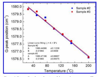
**Figure 5.** Raman G peak as a function of the sample temperature. The measurements were carried out under the low excitation power to avoid local heating while the temperature of the sample was controlled externally. Note an excellent liner fit for the examined temperature range. The obtained dependence is used as a calibration curve for the thermal measurement.
