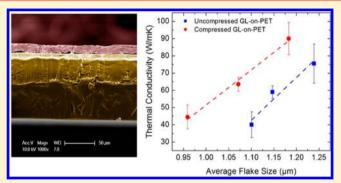
heat conduction than the mass density of the graphene laminate. The thermal conductivity scales up linearly with the average graphene flake size in both uncompressed and compressed laminates. The compressed laminates have higher thermal conductivity for the same average flake size owing to better flake alignment. Coating plastic materials with thin graphene laminate films that have up to  $600 \times$  higher thermal conductivity than plastics may have important practical implications.
