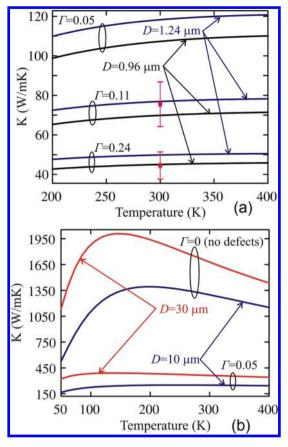
**Figure 8.** Calculated thermal conductivity as a function of temperature shown for different flake size *D* and defect scattering strength  $\Gamma$ . Not that increasing *D* or decreasing  $\Gamma$  increases the thermal conductivity and strengthens its temperature dependence. The experimental data points are shown with the circles.
